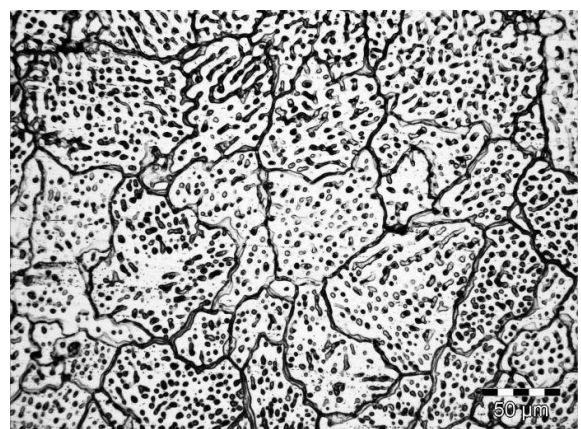
Fig. 1 – Optical micrograph of section of clad produced by 7075 powder clad onto 7075 substrate with a cladding speed of 1900 mm/min and a power of 2378 W, with a Gaussian spot size of 3 mm, taken parallel to the individual track directions; a –as clad; b – heat treated
